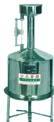
LT-1 标准金属量筒 Standard Metal Measuring Can 不锈钢 stainless steel
